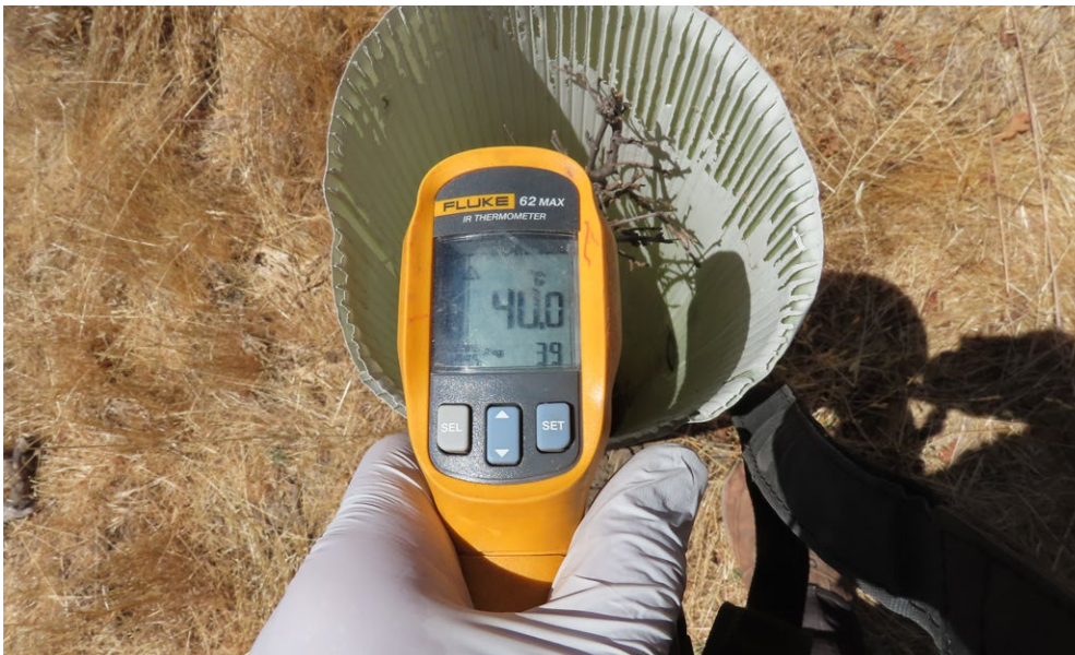
Figure 30—In unshaded sites, temperatures within tree shelters can be well above ambient air temperatures near midday. Temperatures measured by an infrared thermometer within this and other shelters were about 40 °C (104 °F), whereas the ambient air temperature was around 30 °C (86 °F). If plants within shelters are water stressed, they are not able to cool via evapotranspiration, and on hot days, high temperatures in the shelters can scorch or kill leaves. Photo by Tedmund Swiecki.
