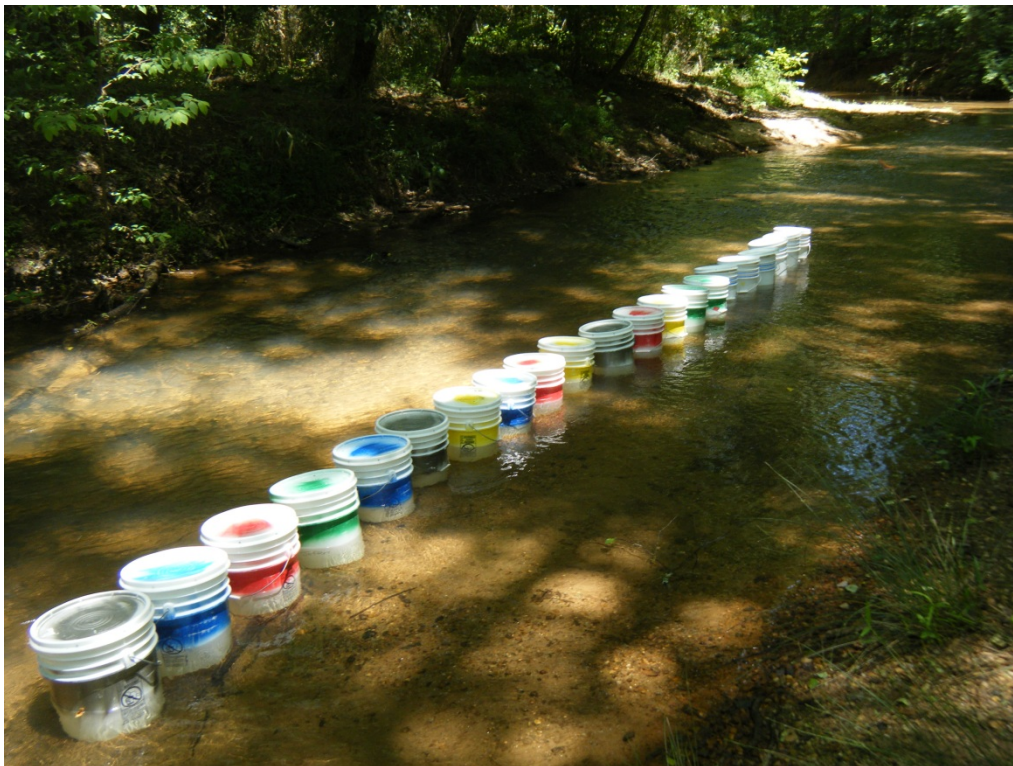
Figure 1—Twenty-one buckets, each containing 10 L of stream water treated with an algaecide or not treated (control), sitting in a stream to maintain ambient water temperature. Fifteen buckets were used to compare efficacy of four algaecides and a non-treated control, and six buckets were used to evaluate reduced rates of one algaecide. Three replicate buckets were used for each treatment, and buckets were arranged in a completely randomized design.
